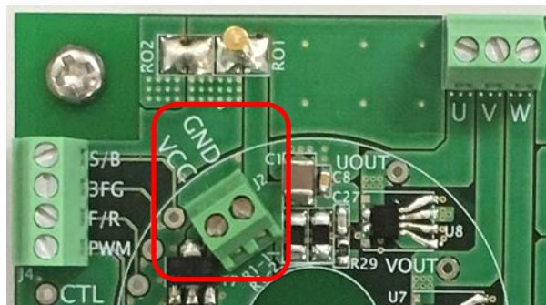
Figure 3. DC power supply connector
