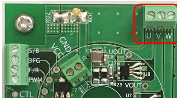
Figure 2. Motor winding Connector
