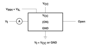
Figure 4. On-State Switch Leakage-Current Test Circuit
