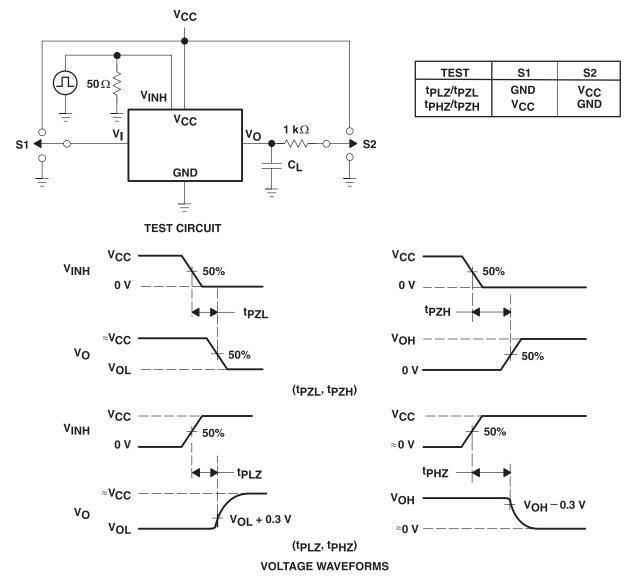
Figure 6. Switching Time (t<sub>PZL</sub>, t<sub>PLZ</sub>, t<sub>PZH</sub>, t<sub>PHZ</sub>), Control to Signal Output
