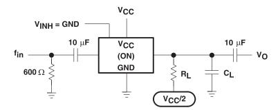
Figure 10. Sine-Wave Distortion
