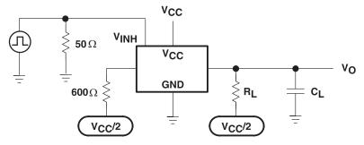
Figure 8. Crosstalk (Control Input, Switch Output)
