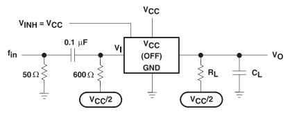
Figure 9. Feedthrough Attenuation (Switch Off)
