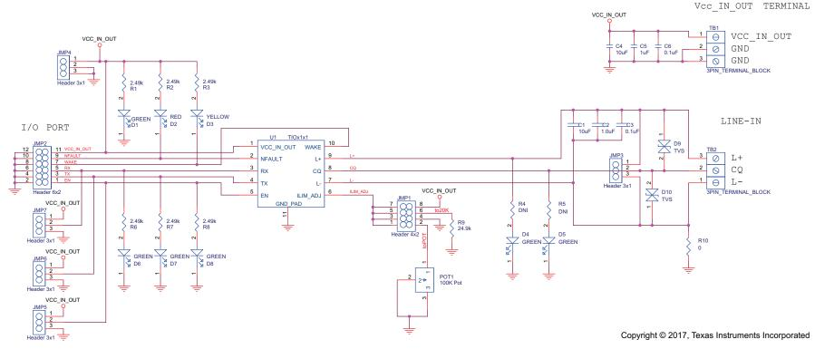
Figure 3. TIOL111-5 and TIOS101-5 EVM Schematic
