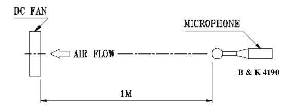
Noise is measured under Rated Voltage in free air in the anechoic chamber with B & K Nexus 4350 conditioning amplifier, with B & K 4190 microphone at a distance of one meter from the fan intake. The background noise is 18dBA max under the ISO-3745 Standard.
