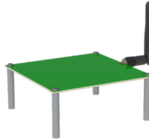
Bent 90°, on edge of ground
