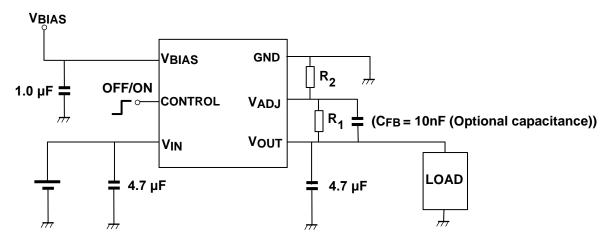
Adjustable Output Voltage ( $V_{OUT} = 0.6 \text{ V}$  : R1 = 0  $\Omega$ , R2 < 4 M $\Omega$ )
