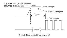
Figure 3. Startup Timing (OE/ST Mode)
