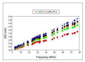
Figure 7. IDD vs Frequency
