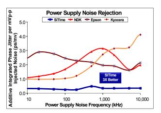
Figure 4. Power Supply Noise Rejection<sup>[4]</sup>
