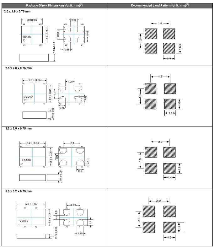
8. Top marking: Y denotes manufacturing origin and XXXX denotes manufacturing lot number. The value of "Y" will depend on the assembly location of the device. 9. A capacitor of value 0.1 µF between Vdd and GND is required.
