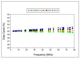
Figure 11. Duty Cycle vs Frequency
