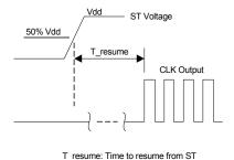
Figure 4. Standby Resume Timing (ST Mode Only)
