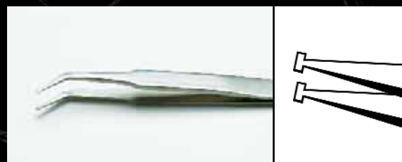
4 1/2" 115mm for handling and positioning 2 and 3 lead SOT packages at 45° angle
