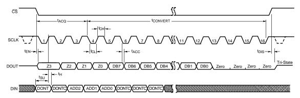
Figure 4. ADC082S021 Serial Timing Diagram
