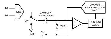
Figure 46. ADC082S021 in Track Mode
