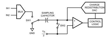
Figure 47. ADC082S021 in Hold Mode
