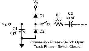
Figure 50. Equivalent Input Circuit
