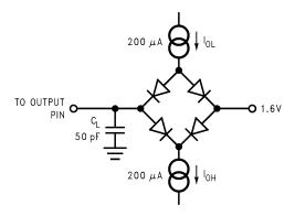
Figure 3. Timing Test Circuit
