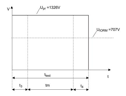
$t_3, t_4 = 0.1 \text{ sec}$  $t_{m(PARTIAL\ DISCHARGE)}$ = 1.0 sec  $t_{test} = 1.2 sec$
