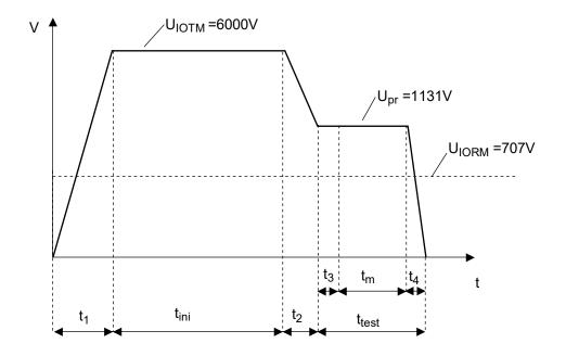
$t_1, t_2 = 1 \text{ to } 10 \text{ sec}$  $t_3, t_4 = 1 \text{ sec}$  $t_{m(PARTIAL\ DISCHARGE)}$ = 10 sec  $t_{test}$  = 12 sec
