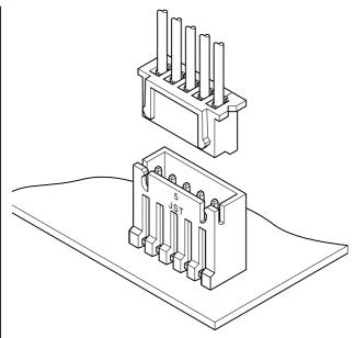
XH connector high box type, with 17.0mm mounting height and with 5.8mm thickness.
