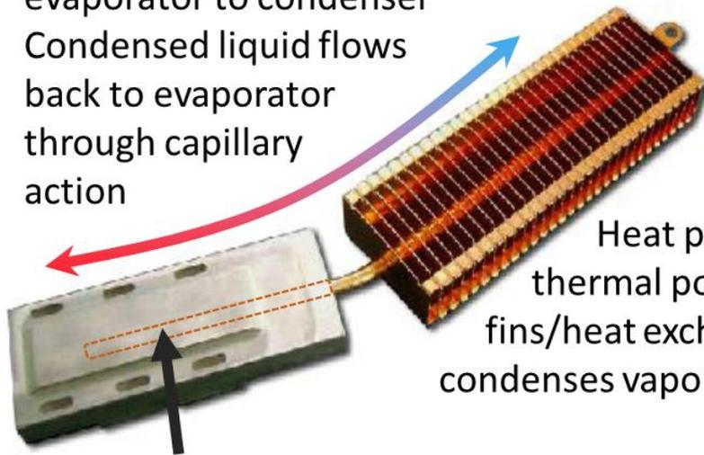
Heat pipe dissipates thermal power to fins/heat exchanger and condenses vapor to liquid
