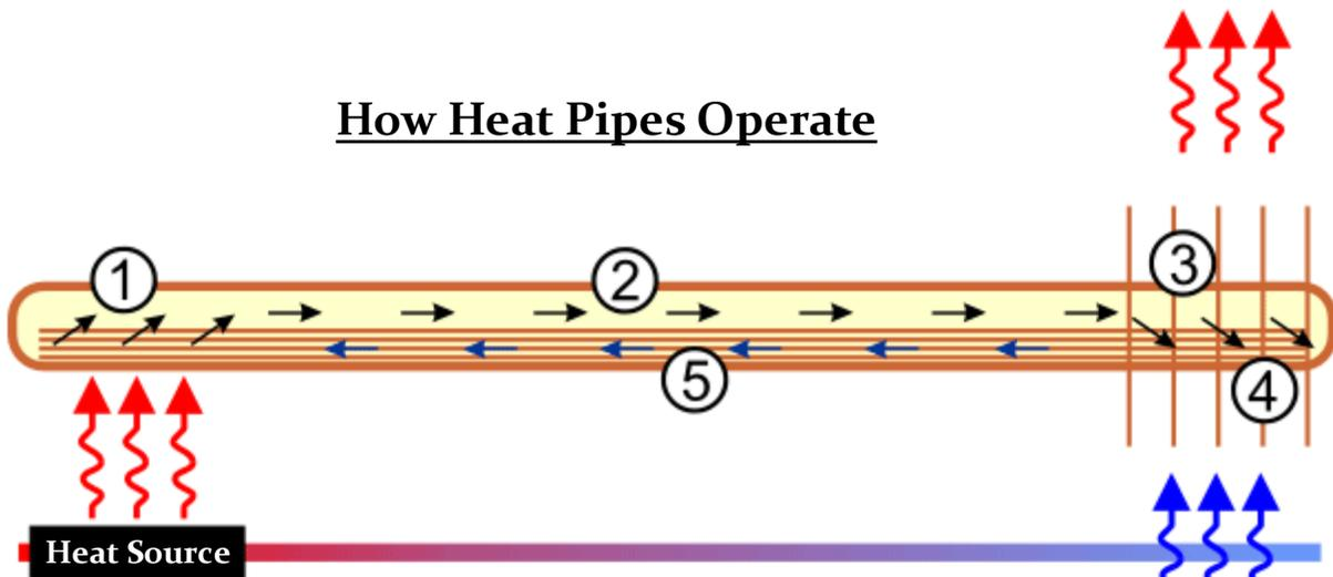
1. Working fluid absorbs heat while evaporating to vapor
