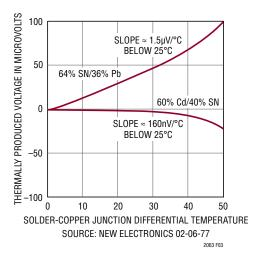
Figure 3. Solder-Copper Thermal EMFs
