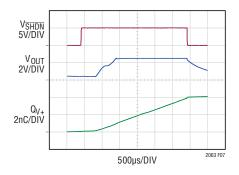
Figure 7. LTC2063 Charge Loss Due to Enabling and Disabling via SHDN Pin
