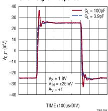
Small Signal Overshoot vs Load Capacitance
