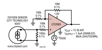
Figure 9. Micropower Precision Oxygen Sensor
