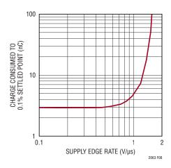
Figure 8. LTC2063 Power-Up Charge vs Supply Edge Rate
