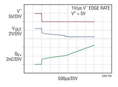
Figure 6. LTC2063 Charge Loss During Power-Up
