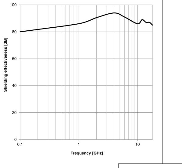
CHECKED REVISION DATE (YYYY-MM-DD) GENERAL TOLERANCE PROJECTION METHOD ViMa 005.003 2020-03-06 DIN ISO 2768-1m DESCRIPTION **WE-LT Conductive Shielding** Würth Elektronik eiSos GmbH & Co. KG Gasket ORDER CODE EMC & Inductive Solutions Max-Eyth-Str. 1 3021310 74638 Waldenburg Germany SIZE/TYPE STATUS Tel. +49 (0) 79 42 945 - 0 www.we-online.com BUSINESS UNIT PAGE WÜRTH ELEKTRONIK 2/3 eiSos Valid Square eiSos@we-online.com
