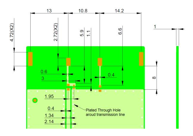
Recommended test board PCB layout for electrical characteristic measurement. Substrate material FR4.
