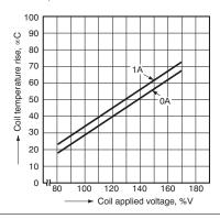
5-(2). Coil temperature rise (200 mW Standard type) Tested sample: HY1Z-12V, 5 pcs.
