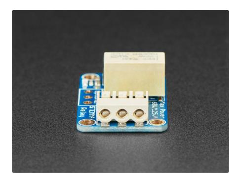
You can switch up to 2A of resistive current at 30VDC or ~40VAC or lower. At 110VDC you can switch up to 0.6A, at 120VAC up to 0.5A, and at 250VAC you can switch up to 0.3A. Check the datasheet for the relay for the exact switching capacity, and of course, for reactive/inductive loads you will need to de-rate. This isn't a relay you can use to turn on and off your washer/dryer, stick to 60W or less.
