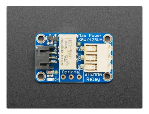
No worrying about flyback diodes, level shifting, pin protection. The STEMMA board takes care of all that for you. You can use it with any 3V or 5V microcontroller/
