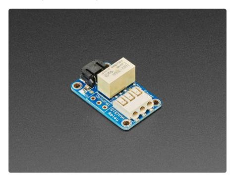
Each STEMMA board comes with a fully assembled and tested PCB but no cable. No soldering is required to use it. There's an optional second switch on the side of the PCB, if you get a 3-pin terminal block (https://adafru.it/GA3) you can solder that in place, but its optional.
