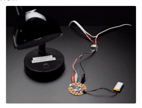
STEMMA plug-and-play parts make your next project solder-free! This is the STEMMA Non-Latching Mini Relay. It gives you power to control, and control over power. Put simply, you can now turn on and off lamps, fans, solenoids, and other small appliances that run on up to 250VAC or DC power using any microcontroller or microcomputer, with ease.
