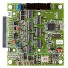
When connected to a DC9003A-C Evaluation/Development Mote, the DC9006 Eterna interface card provides a USB connection for both power and software access to the mote API UART port.
