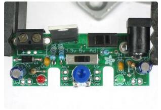
Next we will solder in the 2-pin terminal jack. This lets us connect up wires to power the board from a battery or similar.
