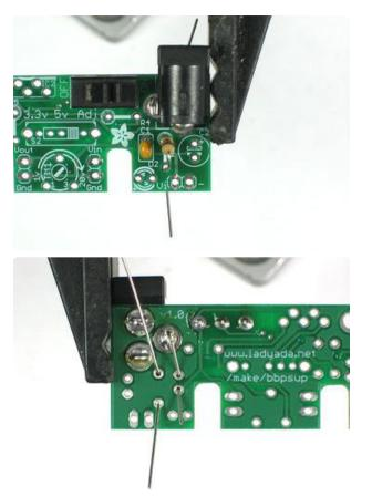
Place one of the 1.0K resistors (Brown Black Red Gold) into the slot marked R1. Then place right next to it one of the 0.1uF ceramic capacitors (they're small and yellow). The resistors and ceramic capacitors are non-polarized so they can go in 'either way'.
