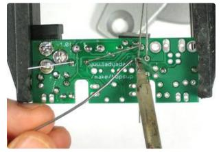
Solder and clip the three resistors.
