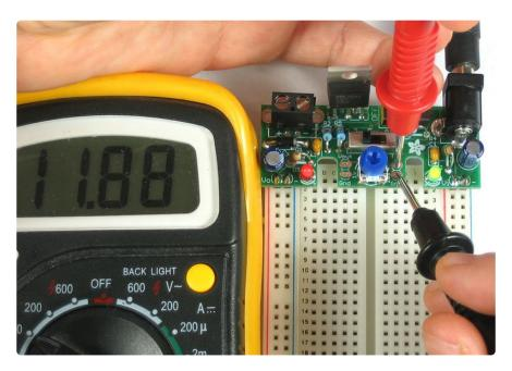
For example, this photo is me testing the output of the right hand side with a 12VDC regulated power adapter attached. The voltage is within 200mV of 12V. The green LED indicates that there is power on the right hand side.
