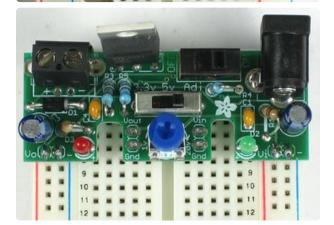
Now place the power supply on top. If it fits nicely, solder the four pins.
