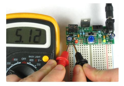
Finally, by selecting Adj. you can adjust the supply to anything you want from as low as  $^{\sim}1.3V$  to within half a volt of the input (which can be as high as 20V).
