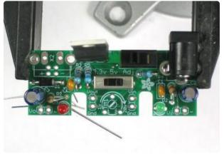
Finish off the 'low voltage' side by inserting the second 1.0K resistor R2 and the second 0.1uF ceramic capacitor C4.
