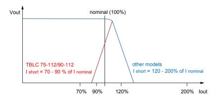
The load characteristic is designed to accomplish reliable start-up of heavy loads.
