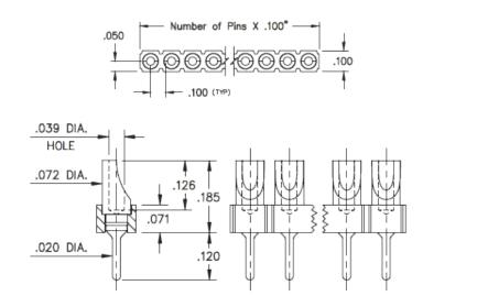
**Description:** Interconnect Header Solder Tail Pin Header SolderCup Head Single Row Through Hole Plating Code: 10 Shell Plating: 10  $\mu$ " Gold over 100  $\mu$ " Nickel
