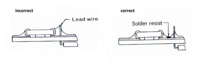
(2) Placing close to chassis.
