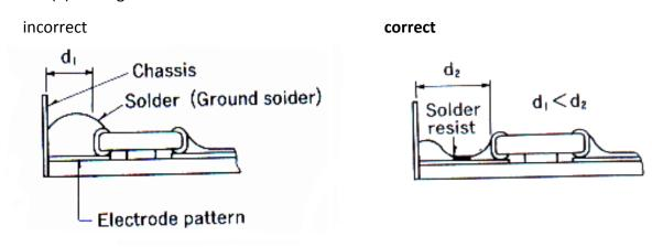
(3) Placing leaded components after chip component.
