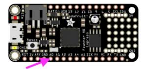
A0 is located between GND and A1 on the opposite side of the board from the battery connector, towards the end with the Reset button.
