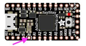
A0 is located between VHI and A1, near the "A" in "Adafruit", and the pin pad has left and right white parenthesis markings around it.
