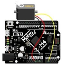
For the Metro M4 Express, ItsyBitsy M4 Express and the Feather M4 Express, connect the ground wire to any G or GND, the power wire to USB or 5V, and the signal wire to A1.
