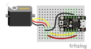
For example, to wire a servo to **Trinket**, connect the ground wire to **GND**, the power wire to **USB**, and the signal wire to **0**.
