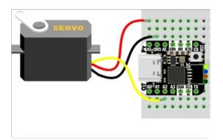
For QT Py M0, connect the ground wire to GND, the power wire to 5V, and the signal wire to A2.
