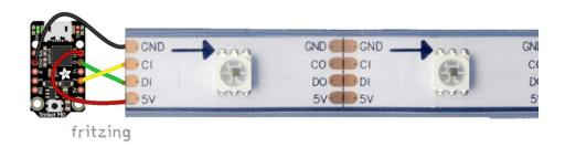
Note that the wire ordering on your DotStar strip or shape may not exactly match the diagram above. Check the markings to verify which pin is DIN, CIN, 5V and GND
