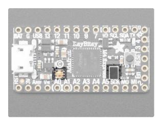
As part of the 'Express' series of boards, this ItsyBitsy is designed for use with CircuitPython. To make that easy, we have added two extra parts: a mini DotStar (RGB LED) and a 2 MB QSPI (Quad SPI) Flash chip
