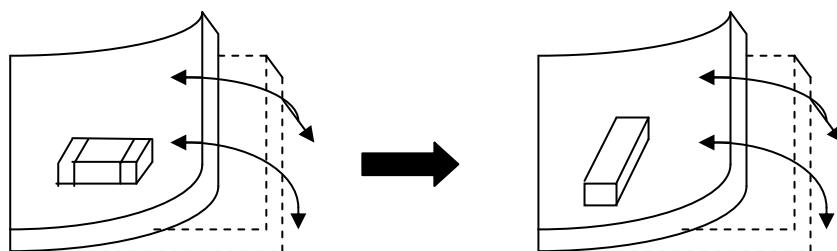
(2) Component layout close to board separation point.
