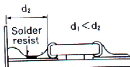
(3) Placing leaded components after chip component.
