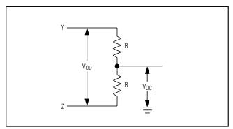
Figure 5. Driver DC Test Load
