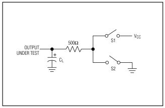
Figure 8. Driver Enable/Disable Timing Test Load
