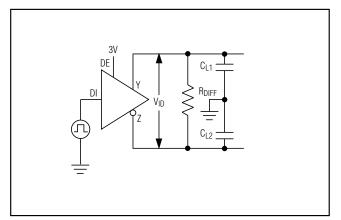
Figure 7. Driver Timing Test Circuit
