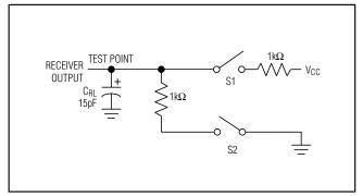
Figure 6. Receiver Enable/Disable Timing Test Load
