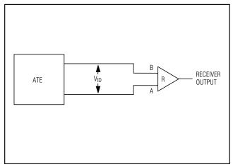
Figure 13. Receiver Propagation Delay Test Circuit
