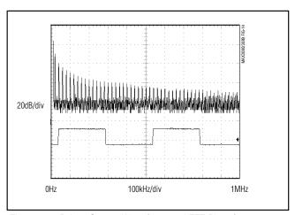
Figure 14. Driver Output Waveform and FFT Plot of MAX3086/MAX3087/MAX3088, and MAX3089 with SRL = GND, Transmitting a 20kHz Signal
