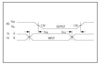
Figure 11. Receiver Propagation Delays
