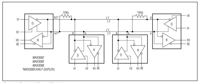
Figure 21. Typical Half-Duplex RS-485 Network
