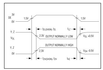
Figure 10. Driver Enable and Disable Times (except MAX3081/MAX3084/MAX3087)
