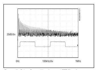
Figure 15. Driver Output Waveform and FFT Plot of MAX3083/MAX3084/MAX3085, and MAX3089 with SRL = V<sub>CC</sub>, Transmitting a 20kHz Signal
