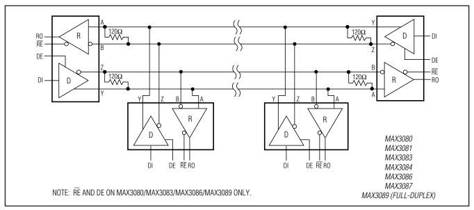
Figure 22. Typical Full-Duplex RS-485 Network
