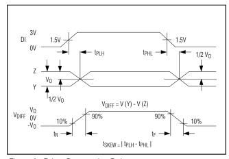
Figure 9. Driver Propagation Delays
