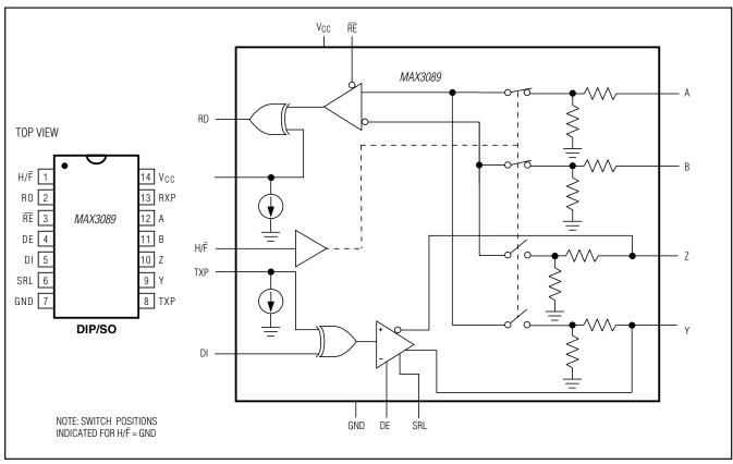
Figure 4. MAX3089 Pin Configuration and Functional Diagram
