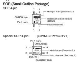
Note: 1. The actual product is marked differently from the image shown here. Note: 2. "G3VM" does not appear in the model number on the Relay. Note: 3. The indentation in the corner diagonally opposite from the pin 1
