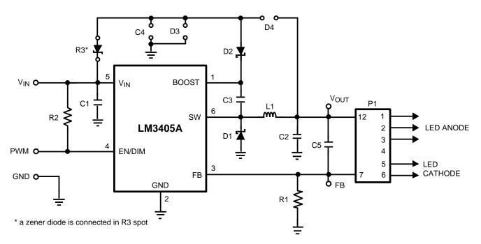
Figure 16.  $V_{BOOST}$  Derived from  $V_{IN}$  through a Series Zener Diode
