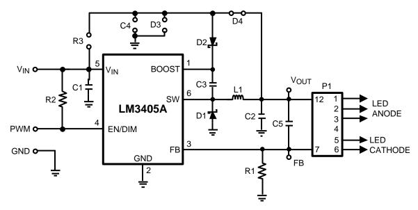
Figure 15.  $V_{\text{BOOST}}$  Derived from  $V_{\text{OUT}}$
