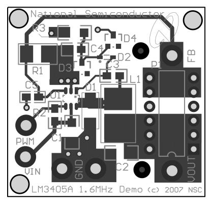
Figure 10. Top Layer and Top Overlay
