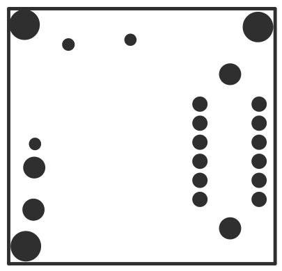
Figure 12. Internal Plane 1 (GND)
