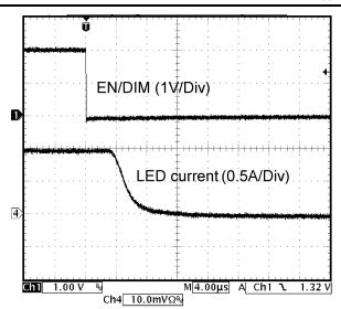
$t~(4\mu s/\text{DIV})$  Figure 9. Shutdown During PWM Dimming  $(V_{\text{IN}}=12~V,\,I_{\text{F}}=1\text{A})$
