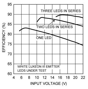
Figure 6. Efficiency vs Input Voltage  $(I_F = 1A)$
