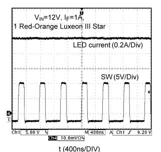
Figure 7. Switching Waveforms
