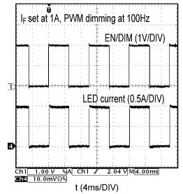
Figure 2. PWM Dimming of LEDs
