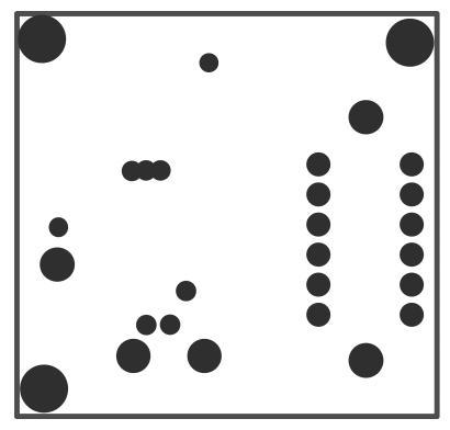
Figure 13. Internal Plane 2 ( $V_{IN}$ )
