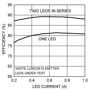
Figure 5. Efficiency vs LED Current  $(V_{IN} = 12 \text{ V})$
