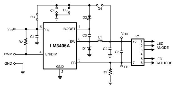
Figure 14.  $V_{BOOST}$  Derived from  $V_{IN}$
