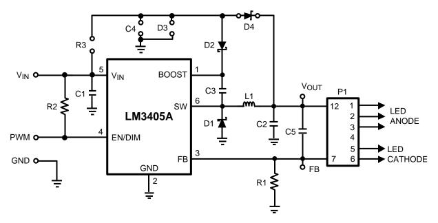
Figure 17.  $V_{\text{BOOST}}$  Derived from  $V_{\text{OUT}}$  through a Series Zener Diode
