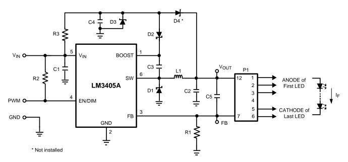
Figure 1. LM3405A Demo Board Schematic
