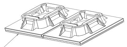
∠ ADHESIVE BACKING: ACRYLIC BASED ADHESIVE PRESSURE SENSITIVE FOAM TAPE 0.04 (1.0) THICK WITH A PROTECTIVE LINER. MOUNT IS DESIGNED TO SUPPORT 0.50 lbs (227g) MAX. WEIGHT ON A CLEAN DRY SMOOTH SURFACE.
