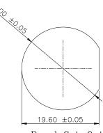
Panel Cut-Out Panel Thick:1.5~2.0mm
