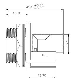
Nut - Torque Spec (0,56 Nm)
