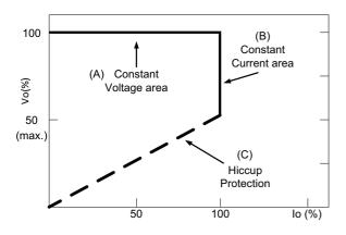
Typical LED power supply I-V curve
