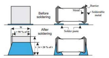
Figure 4: Soldering Criterion in case of Wave and IR Reflow Pb-containing Soldering
