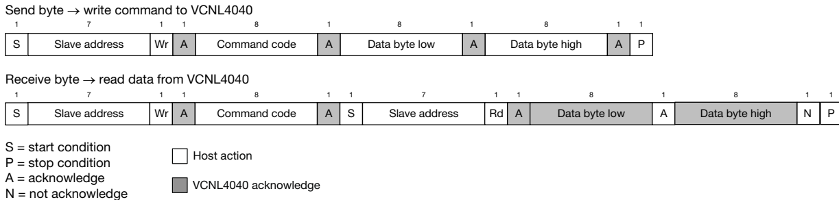
Fig. 12 - Write Word and Read Word Protocol
