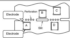
(3) Mounting components near screw holes
