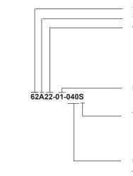
Style: A = 1/2" package, 5.0 Vdc Input, D = high torque w/5.0 Vdc input, V = 3.3 Vdc input
