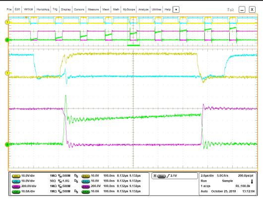
Figure 9-6. SiC MOSFET Switching Waveforms
