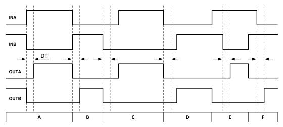
Figure 8-4. Input and Output Logic Relationship With Input Signals
