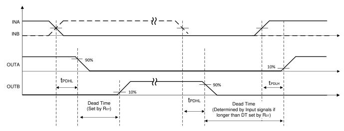
Figure 7-4. Dead-Time Switching Parameters
