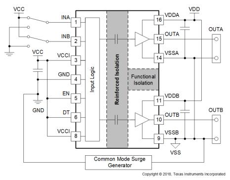
Figure 7-7. Simplified CMTI Testing Setup
