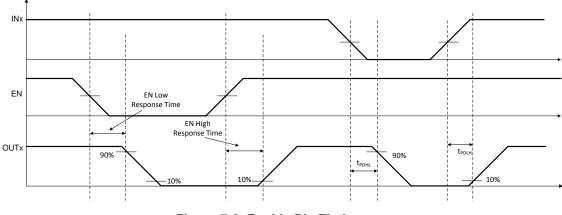
Figure 7-3. Enable Pin Timing
