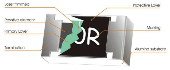
Fig 1. Construction of Chip-R
