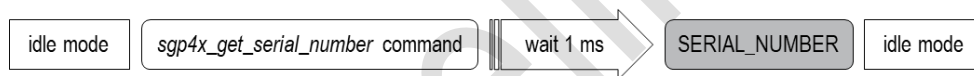
Figure 14 Process flow for reading out the serial number of the SGP41 sensor.
