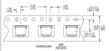
Unless otherwise specified, tolerances in decimals are .X  $\pm$  0.3, .XX  $\pm$  0.15 for lengths in millimeters and  $\pm1$  ° for degrees.
