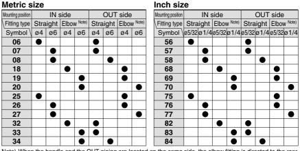
Note) When the handle and the OUT piping are located on the same side, the elbow fitting is directed to the rear side (DIN rail side). Use caution to ensure the connector is not disturbed, depending on piping direction, when choosing to attach a digital pressure switch.
