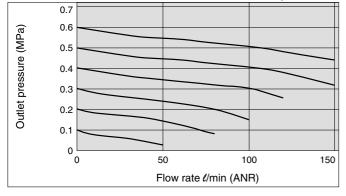
ARM11AA1-310 (One-touch fittings: IN ø8, OUT ø6) Condition: Inlet pressure 0.7 MPa
