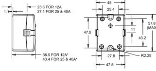
\* Overall height dimensions includes with clear cover Dimensions in mm
