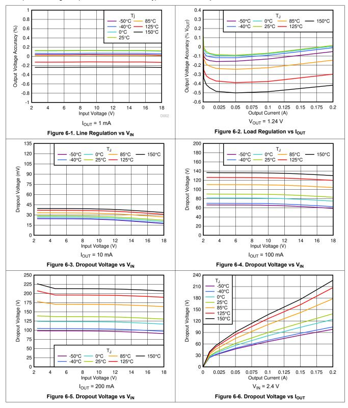
at operating temperature  $T_J = 25^{\circ}C$ ,  $I_{OUT} = 1 \text{ mA}$ ,  $V_{EN} = 0.9 \text{ V}$ ,  $C_{IN} = 2.2 \mu\text{F}$ ,  $C_{OUT} = 2.2 \mu\text{F}$ , and  $V_{IN} = V_{OUT(typ)} + 0.8 \text{ V}$  or 2.4 V (whichever is greater), unless otherwise noted; typical values are at  $T_J = 25^{\circ}C$
