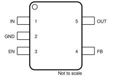
Figure 5-1. DBV Package (Adjustable), 5-Pin SOT-23 (Top View)
