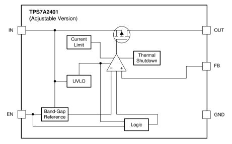
Figure 7-1. Adjustable Version Block Diagram
