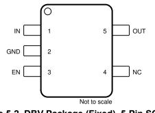
Figure 5-2. DBV Package (Fixed), 5-Pin SOT-23 (Top View)
