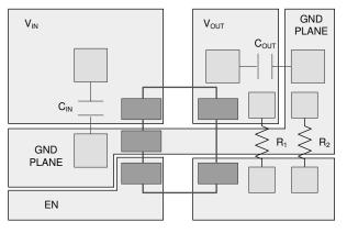
Figure 10-1. Adjustable Version Layout Example
