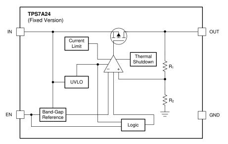
Figure 7-2. Fixed Version Block Diagram
