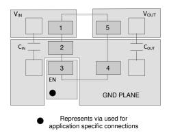
Figure 10-2. Fixed Version Layout Example
