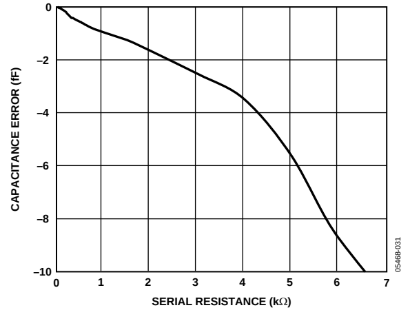
Figure 15. Capacitance Input Error vs. Serial Resistance, C_{IN}(+) to EXC = 21 pF, C_{IN}(-) to EXC = 23 pF, V_{DD} = 5 V, the Same Configuration as in Figure 34.
