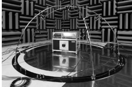
Noise characteristic measurement equipment
