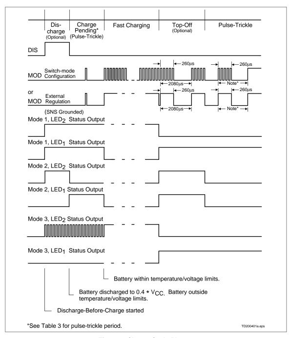
Figure 2. Charge Cycle Phases
