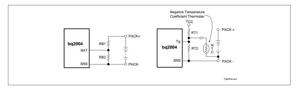
Figure 1. Voltage and Temperature Monitoring
