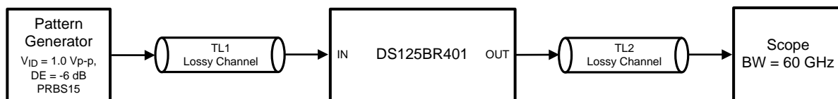
Figure 10. Test Setup Connections Diagram
