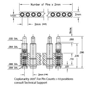
**Description:** Interconnect SLC Header Spring-Loaded Header Vertical Mount SMT Single Row Surface Mount Plating Code: 22 Shell Plating: 20µ" Gold over 100µ" Nickel Inner Spring Plating: 10µ" Gold Packaging: Packaged in Bulk
