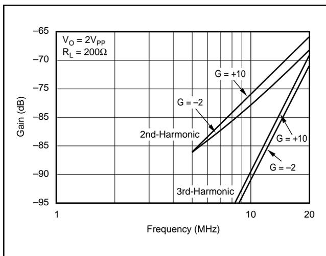
FIGURE 7. Distortion Comparison at  $G = +10$  versus  $G = -2$ .
