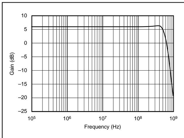
FIGURE 10. Noninverting Gain of +2 Response Using External Compensation.
