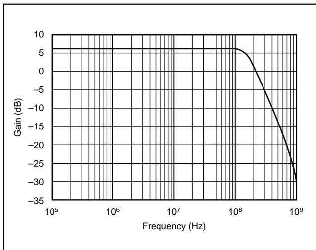
FIGURE 6. Gain of  $-2$  Frequency Response Using External Compensation.
