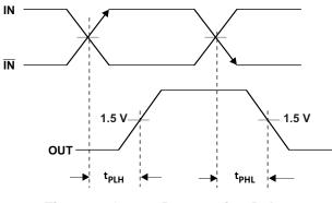
Figure 2. Output Propagation Delay
