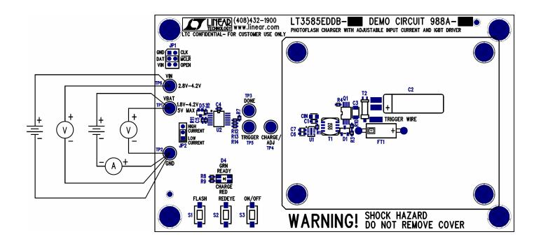
Figure 1. Proper Measurement Equipment Setup
