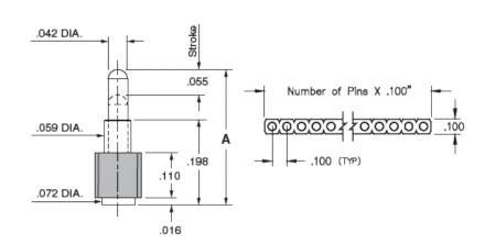
**Description:** Interconnect SLC Header Spring-Loaded Header Vertical Mount SMT Single Row Surface Mount **Plating Code:** Shell Plating: 20μ" Gold over 100μ" Nickel Inner Spring Plating:
